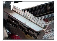
The profile storage magazine provides storage capacity for up to 15 different types of profile bars
