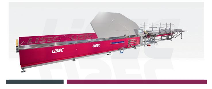
The BSV-45ANK is a fully automatic spacer profile bending machine for processing all conventional, synthetic and composite spacer frames for the production of insulating glass.
